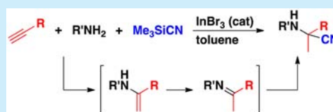
Scheme 1. Strecker-Type Reaction of Ketimines Derived from (a) Ketones and (b,c) Alkynes
